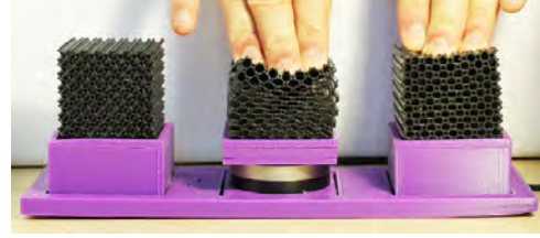
Figure 4: In a single trial participants were presented with three different samples. Their task was to compare softness difference between the leftmost and the rightmost pair. Additionally, we placed a force sensor beneath the middle block in order to collect force data throughout the entire experiment.
